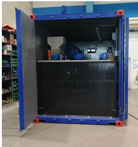
only for visualization: polymer unit of DSE mobile centrifuge decenter ZR15046
